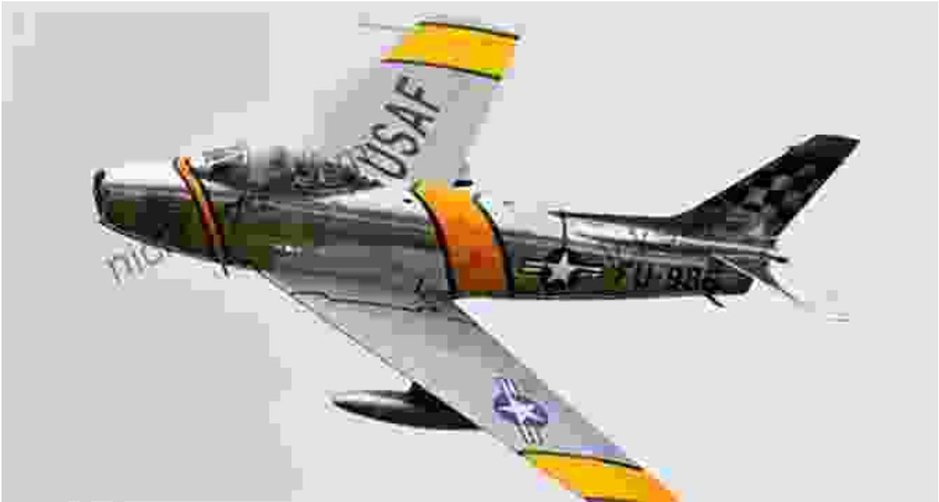
The North American F-86 Sabre Jet revolutionized aerial combat during the Korean War. Its sleek swept-wing design and powerful J47 turbojet engine gave it a significant advantage in speed and maneuverability over its Soviet counterpart, the MiG-15.
